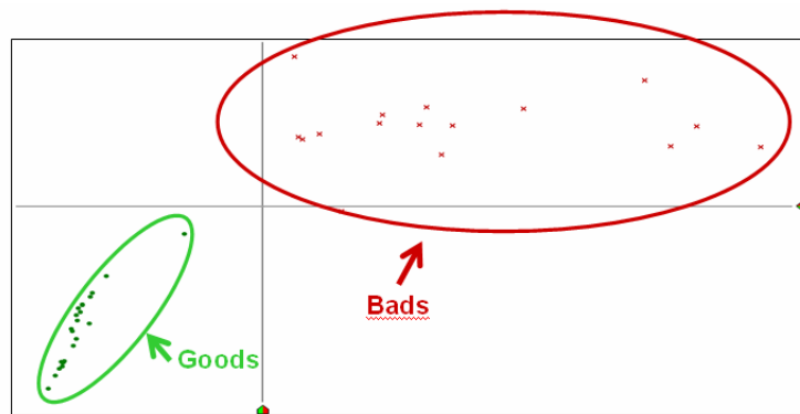
Figure 10 – PCRT sort solution of single crystal blades with part categorization confirmed by X-ray analysis.
