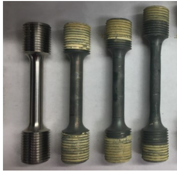
FIGURE 4. Progression of creep in physical dogbones
