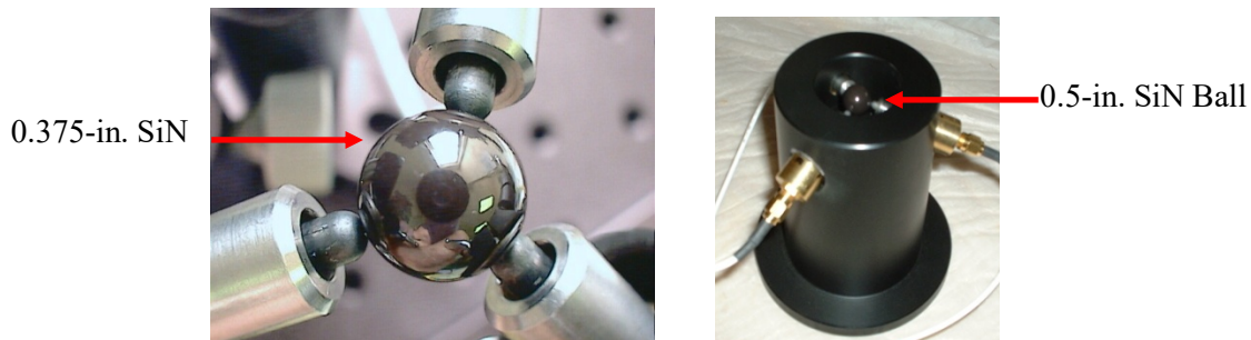
Figure 2. Typical Test Fixtures for Ceramic Balls
