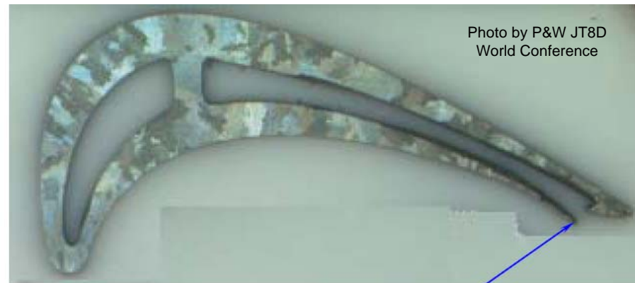
Thin Wall Condition
