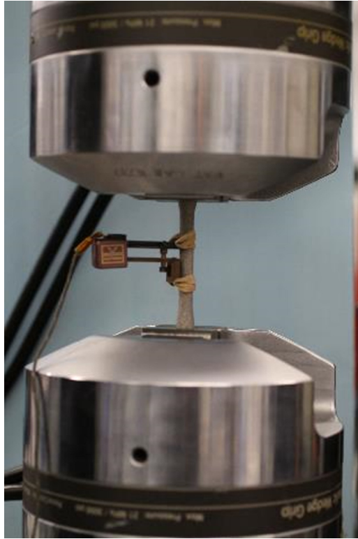
FIG. 11 Tensile testing load cell at Northrop Grumman Mechanical Test Lab holding a CalRAM Ti-6Al-4V ASTM E8 dog-bone test specimen (approved for public release: NG 18-1423 dated July 2, 2018).
