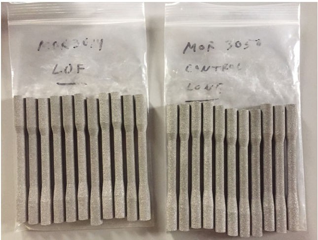
FIG. 13 CalRAM Ti-6Al-4V ASTM E8 dog-bone test specimens.
