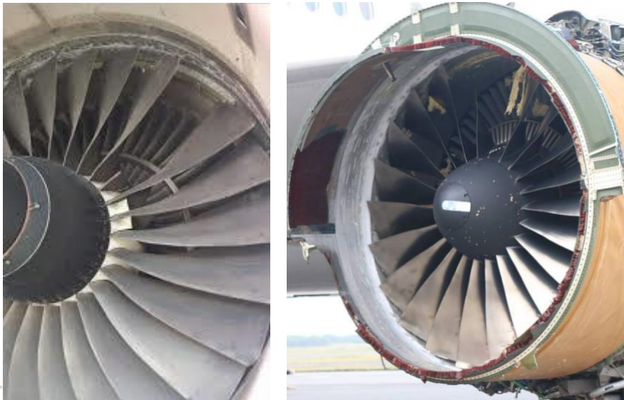
Figure 1 – Image of Air Asia Trent 772 Failure (left) and United PW4077 failure (right).
