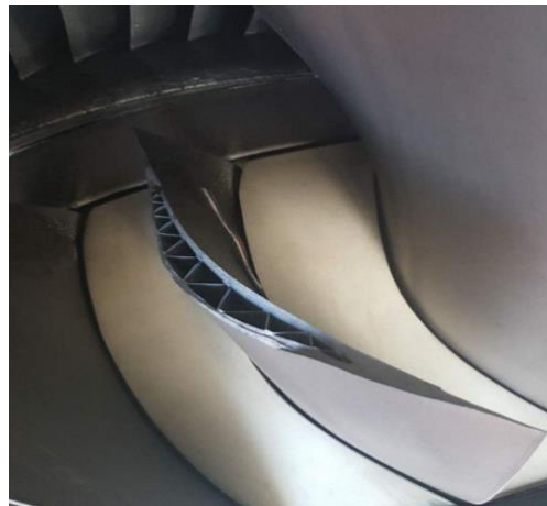
Figure 2 –Close up of Air Asia Trent 772 Failure
