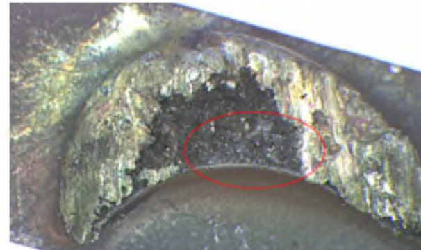
Sinuous interdendritic casting anomaly
