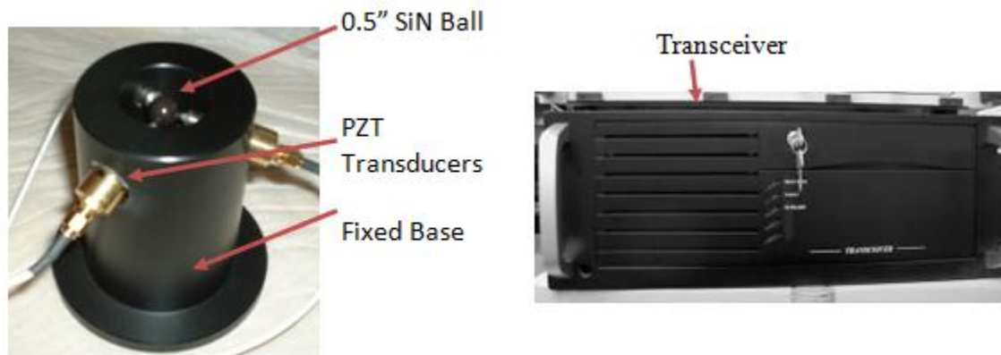
Figure 1 – PCRT fixture for hybrid bearings (left). PCRT transceiver (right).
